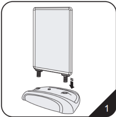
The cartons will contain a water-fill base and a poster frame. Insert the poster frame into the holes in the water fill base.
